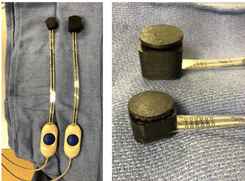
FIGURE 4: Sensors inserted into their respective 3D printed sensor housing. The shorter sensor (left side of left image; bottom of right image) measures thumb CMC force, whereas the taller sensor (right side of left image; top of right image) was used to measure thumb-to-index finger key pinch force.
