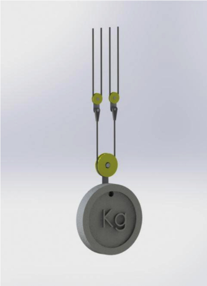
Figure 2. Computer-generated drawing of a force equalization pulley system. The 4 top cables are attached to 4 FDP tendons, 4 FDS tendons, or 4 extensor tendons (or combined extensor tendon units). A single weight produces equal forces on the attached tendons.
